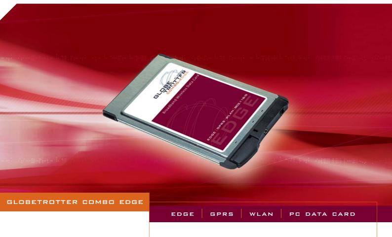
GlobeTrotter COMBO EDGE is the ultimate PC Data Card solution delivering broadband wireless capability to laptops and notebooks by combining EDGE, GPRS, and WLAN technologies in a single PC Card package.
