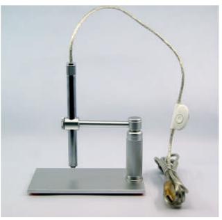
focusing knob on the top while viewing. And the pen microscope can be move up and down for focusing or adjust the size of view by turning the pillar (see the photo) for getting larger photo area or smaller photo area.
