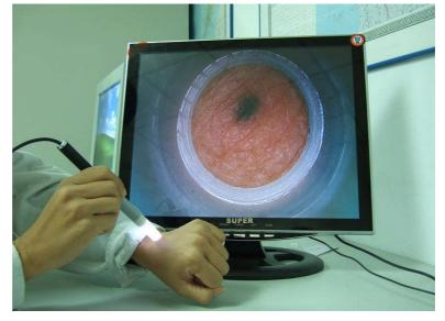
multi-function tube is that it saves you from the need to constantly adjust the focus when you use the pen camera to view parts or flat surface materials and have to constantly move the camera. By attaching a multi-function tube to the pen camera, you can press the tube against the surface of the materials you want to view and thus always maintain a constant distance between the lens of the pen camera and the materials.
