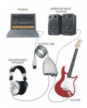
Connect this *USB Guitar Link Cable* to your computer, the LED lights up Gree indicates successful connection. If you'd not like headphone, you can connect a pair of active monitors to the PHONES Connector on the USB Guitar Link Cable.
