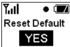
**ENTER:** To unlock the reset default. The background of the characters is reversed. Using **SEL** to select "YES" or "NO". Pressing **ENTER** upon "YES" will restore the factory setting back to GPS DATA LOGGER. Then, the display will be back to normal when it is done.
