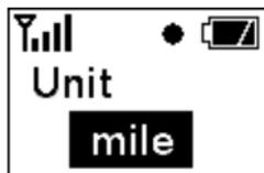
**ENTER:** To unlock the unit setting. The background of the characters is reversed. Using **SEL** to change the unit. Pressing **ENTER** again to confirm the selection and the display will be back to normal.
