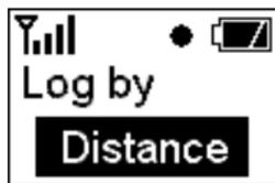
**ENTER**: To unlock the log mode setting. The background of the characters is reversed. Using **SEL** to change log mode. Pressing **ENTER** again to enter the sub-menu for parameter setting.
