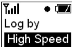
**ENTER**: To unlock the log mode setting. The background of the characters is reversed. Using **SEL** to change log mode. Pressing **ENTER** again to confirm the selection and the display will be back to normal.
