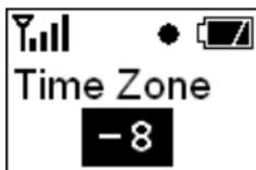
**ENTER:** To unlock the time zone setting. The background of the characters is reversed. Using **SEL** to change the time zone. Pressing **ENTER** again to confirm the selection and the display will be back to normal.
