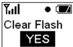
**ENTER:** To unlock the clear flash. The background of the characters is reversed. Using **SEL** to select "YES" or "NO". Pressing **ENTER** upon "YES" will clear the whole storage with all its log data. Then, the display will be back to normal when it is done.
