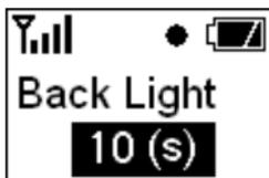
**ENTER**: To unlock the LCD back light timer setting. The background of the characters is reversed. Using **SEL** to change the timer value. Pressing **ENTER** again to confirm the selection and the display will be back to normal.
