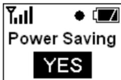
**ENTER:** To unlock the power saving setting. The background of the characters is reversed. Using **SEL** to change the power saving mode. Pressing **ENTER** again to confirm the selection and the display will be back to normal.
